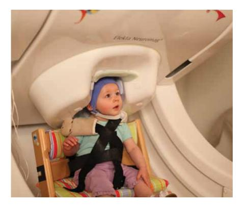
Figure 2 Infant in a MEG machine during measurement.
